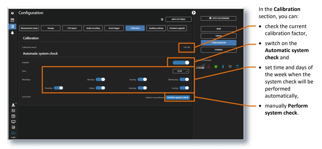
When **Automatic system check** is enabled the calibration factor of the instrument will be periodically verified using the built-in speaker.
