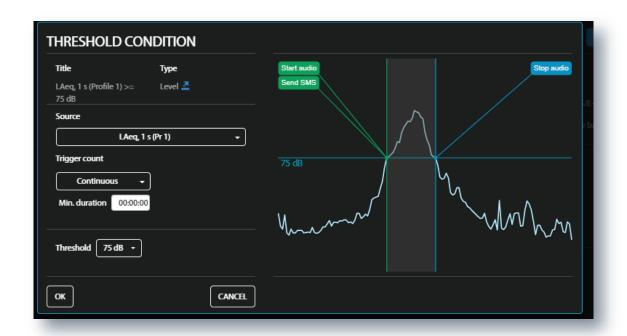
The Threshold type trigger activates the event when some result (Source) exceeds the Threshold level under Trigger count condition: if Trigger count is Continuous, exceeding the threshold level must last longer than Min. duration or such exceeding will be repeated at least several times (1 time, 2 times, ... 10 times).
