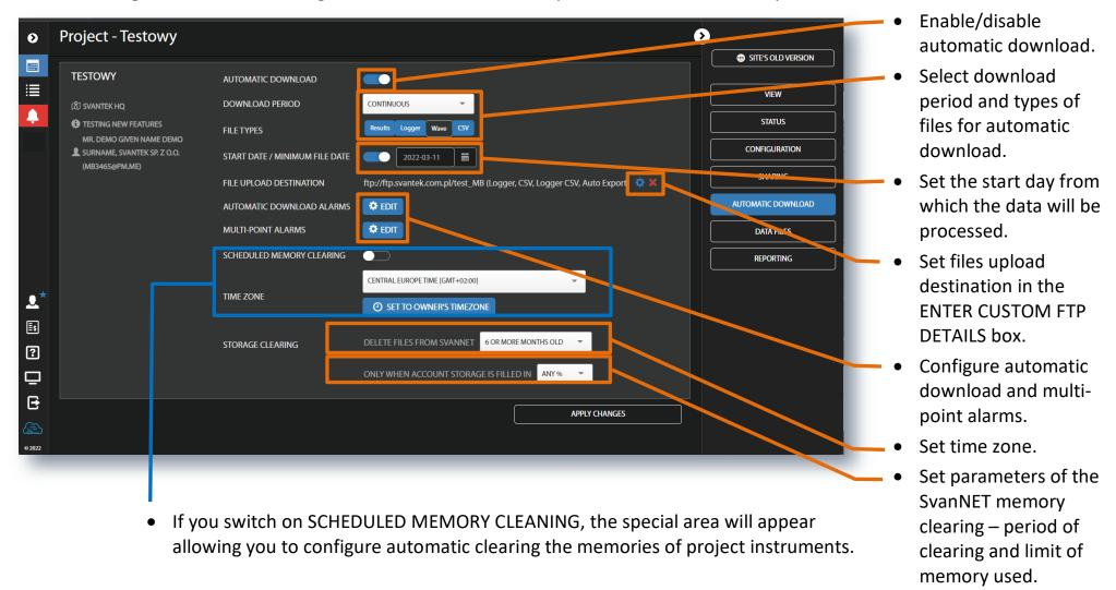
In the ENTER CUSTOM FTP DETAILS section, you can define the parameters for connecting to the FTP / SFTP server and what results will be sent to it. In detail it is described in Appendix B.
