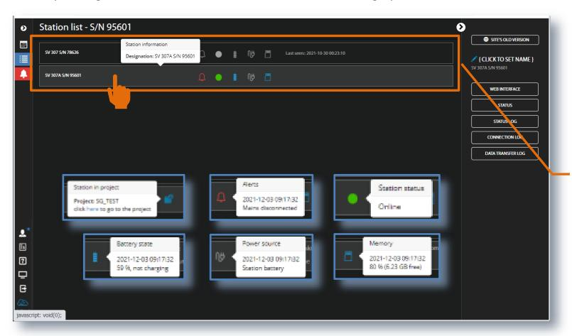
The station bar except the station name and its serial number includes five or six icons that indicate station states. When the station is disconnected from SvanNET all icons are of grey colour.
