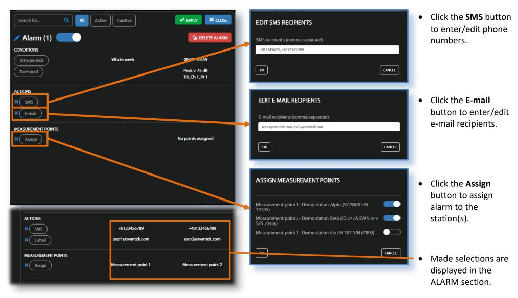
Multi-point alarms are generated when several automatic download or instrument alarms occur within specified time interval.
