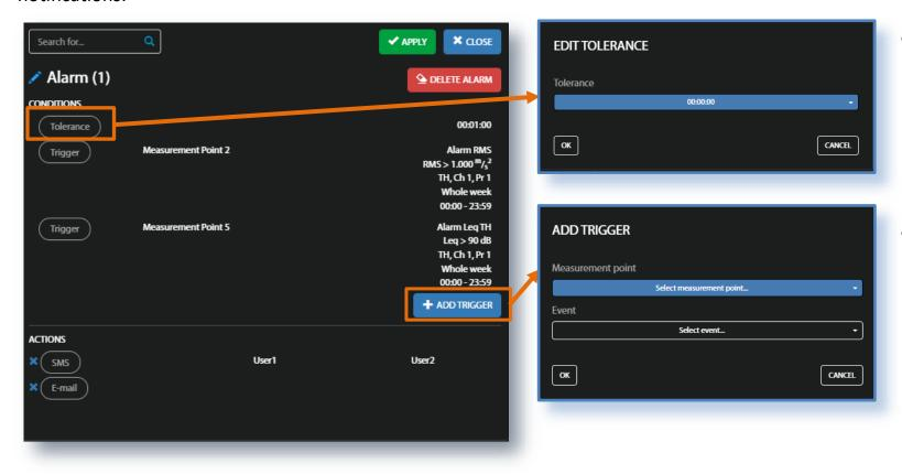
Click the Tolerance button to select in the EDIT TOLERANCE pop-up box the time interval during which multi-point events will be considered.
