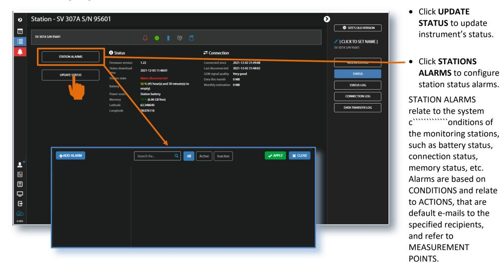
Click **+ADD ALARM**, to configure CONDITIONS, ACTIONS and MEASUREMENT POINTS settings. Alarm CONDITIONS can be defined in the EDIT CONDITION box, opened when you click the **Status** button.
