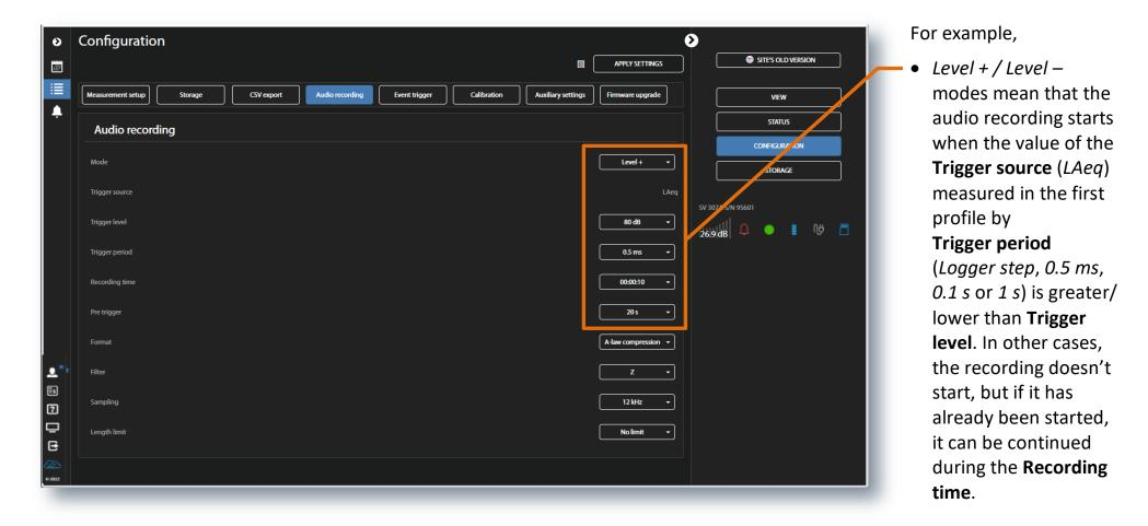
If during the **Recording time** a trigger condition appears, the recording will be prolonged for another **Recording time** from the moment of that trigger condition and so on. If during next recording time there are no triggers, the recording will be stopped after the last trigger plus **Recording time**.
