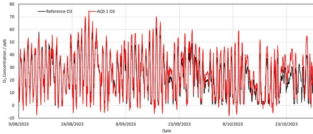
**Figure 4:** Hourly time series data for AQS 1 and Thermo Scientific Ozone Analyzer from August 9<sup>th</sup> to October 30<sup>th</sup>, 2023, for the Calgary Inglewood station.
