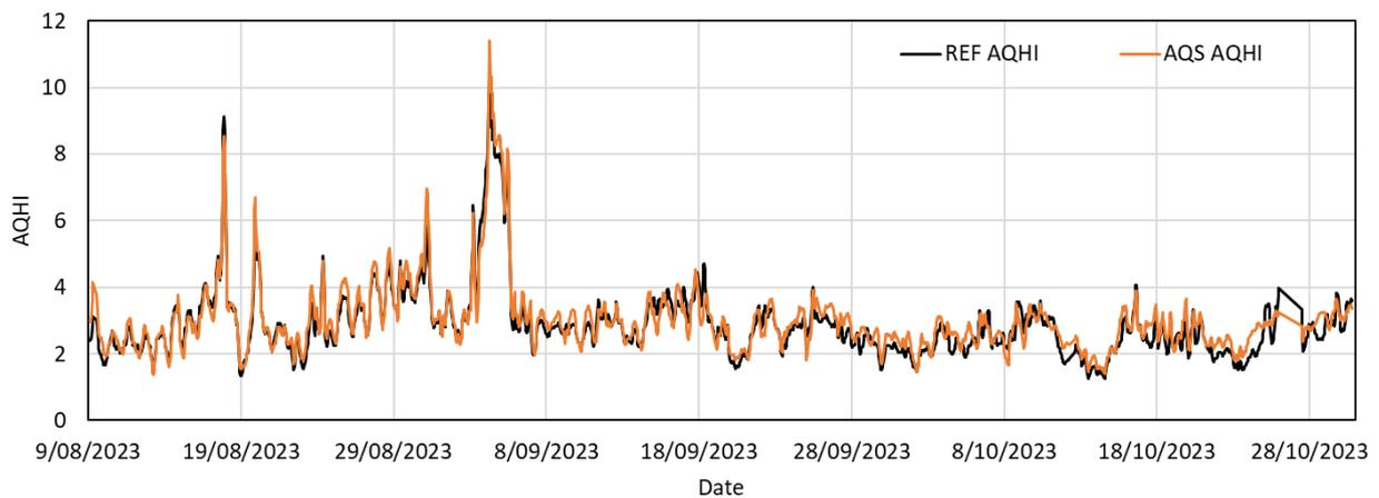
**Figure 13:** Hourly AQHI calculated using the AQS 1 data and the reference station data from August 9<sup>th</sup> to October 30<sup>th</sup>, 2023, for the Calgary Inglewood reference station.
