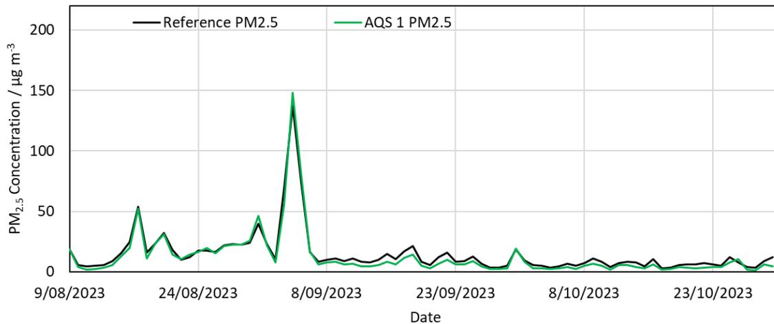
**Figure 10:** 24-hour time series data showing AQS 1 PM<sub>2.5</sub> data and the Teledyne T640 PM<sub>2.5</sub> data from August 9<sup>th</sup> to October 30<sup>th</sup>, 2023, for the Calgary Inglewood reference station.
