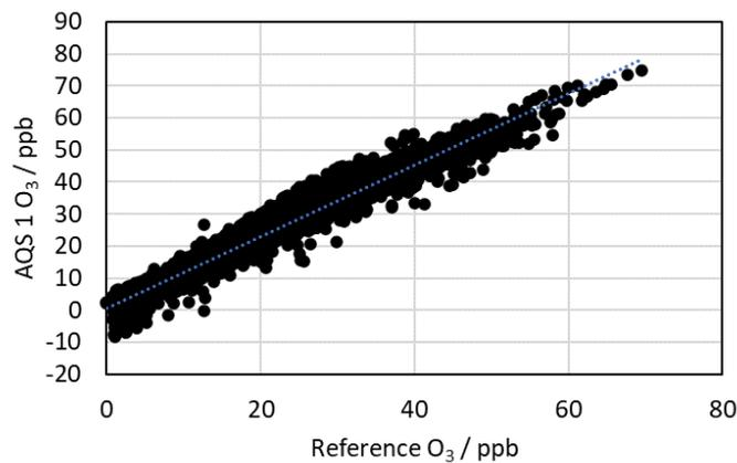
**Figure 5:** Scatter plot comparing hourly AQS 1 ozone module and Thermo Scientific Ozone Analyzer data for the Calgary Inglewood station from August 9<sup>th</sup> to October 30<sup>th</sup>, 2023.
