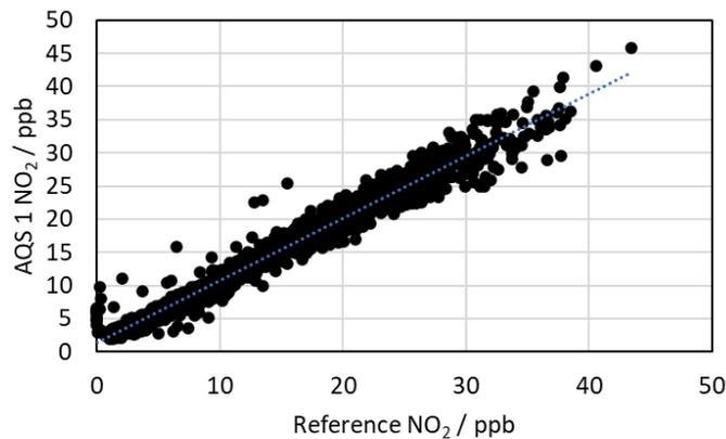
**Figure 8:** Scatter plot comparing hourly AQS 1 NO<sub>2</sub> module and Thermo Scientific NO-NO<sub>2</sub>-NO<sub>x</sub> Analyzer data for the Calgary Inglewood station from August 9<sup>th</sup> to October 30<sup>th</sup>, 2023.
