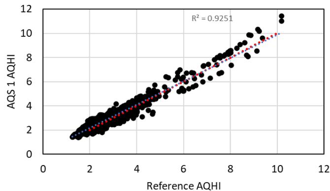
**Figure 14:** Scatter plot comparing the AQHI calculated using the reference data and AQHI calculated using the AQS 1 data for August 9<sup>th</sup> to October 30<sup>th</sup>, 2023, for the Calgary Inglewood reference station. The coefficient of determination is 0.9251. The blue dashed line is the fitted regression line and the red dashed line is the 1:1 line.
