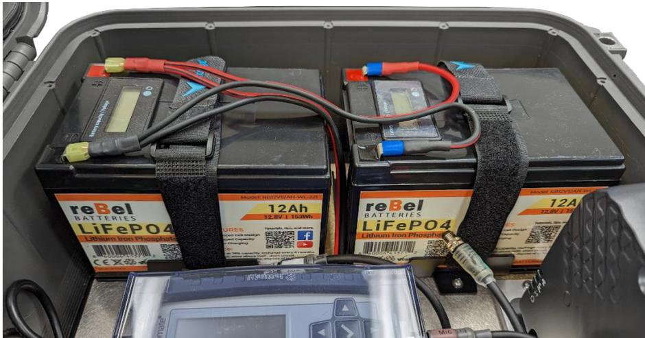
3. Once your batteries are installed, switch the charging switch to ON, then turn system power to ON
