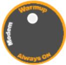
Use the Always ON mode when troubleshooting or configuring the unit initially to allow remote access. Then if needed switch back to Warmup. Use of the Modem Warmup feature can triple the battery life of the Powermate system.
