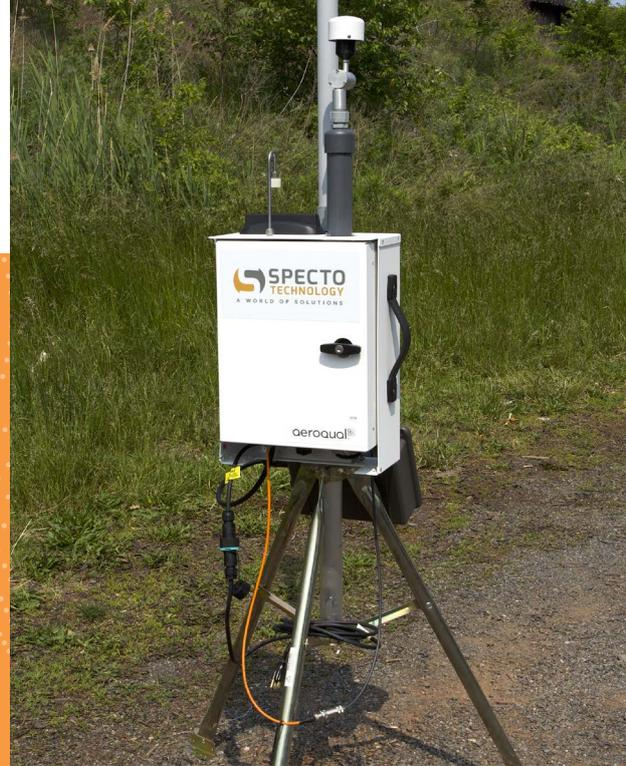
We've designed a NYSDEC DER-10 CAMP Monitoring package using the latest in hardware and software technology to make monitoring easy. Weatherproof monitors arrive fully assembled, with tripod, 15-hour lightweight battery pack and connection to Aeroqual cloud for automated data collection, presentation, alerts and PDF reporting.
