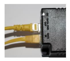
To power the Edge Repeater using this method, a standard Ethernet cable with RJ45 connectors must be connected to the Edge Repeater on one side, and to the DATA & Power OUT port of the PoE injector.
