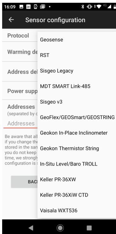
Figure 45, List of protocols compatible with LS-G6-DIG node
