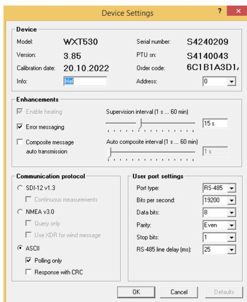
3. Set the sensor in Modbus mode (see chapter 4.10 Changing from CLI mode to Modbus mode from the Vaisala user guide). It is important to ensure that the sensor has changed to Modbus mode. This can be checked by opening the Configuration Tool and testing that there is no communication with the sensor.
