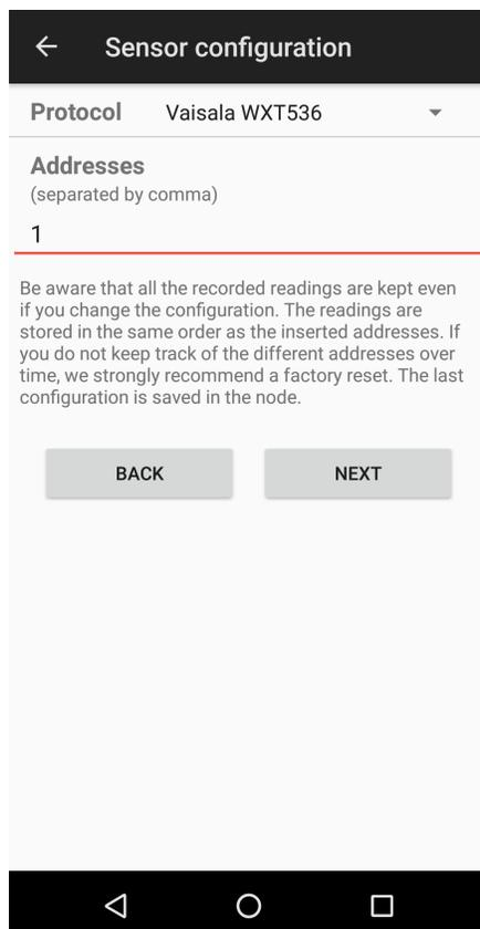
Figure 48, Bus address of the digital sensors
