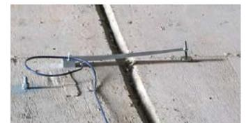
Model 4420-3 Low Profile Crackmeter for measurements in the "Z" direction.
