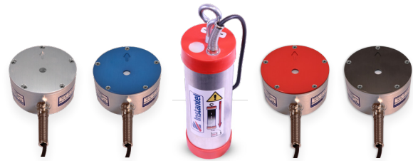
Triaxial geophones configured to international compliance standards. From left to right: ISEE, DIN, ISEE/DIN borehole, Swedish Pile Driving, Swedish Blasting.
