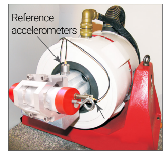
ISEE borehole geophone mounted on a shake table with reference accelerometers.
