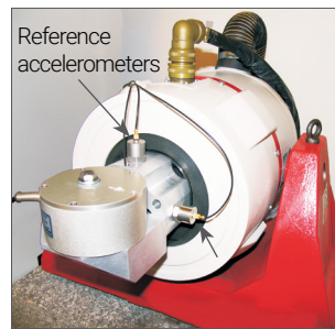
ISEE geophone mounted on a shake table with reference accelerometers.
