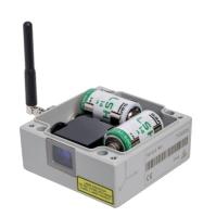
The LaserTilt90 wireless sensor is a 2-in-1 laser distance meter and tiltmeter. The laser measures the relative distance between pairs of reference points. One of the two points can be a natural surface or target foils while the node can be placed at the other end point. Meanwhile, the tiltmeter provides measurements of changes from the vertical level, either on the ground or in structures and is used to monitor inclinations, movements and differential settlements of slopes or infrastructures.
