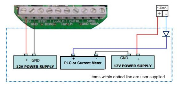
Note: The 4-20mA outputs are located on the side of the unit
