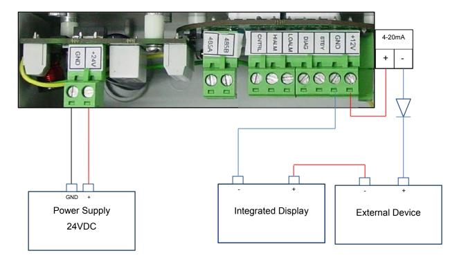
Note: The integrated display is a single ended device and therefore always needs to be located at the end of the loop.
