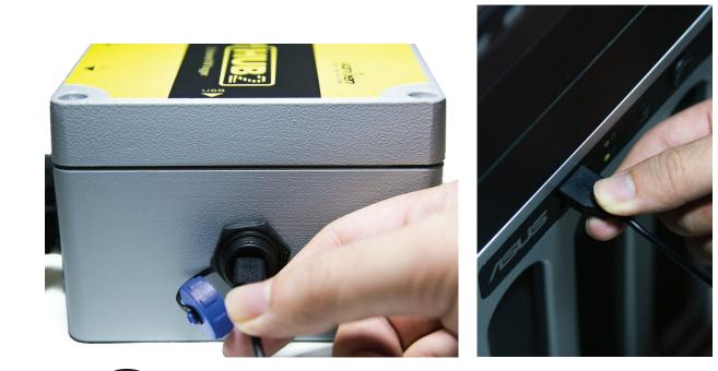
Connect the USB cable to the blue caped port of the VW HUB2 and to the USB port of your computer.
