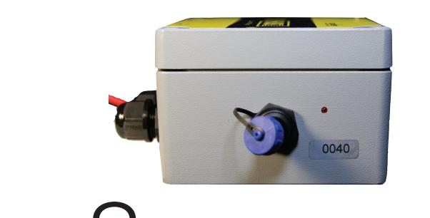
Screw the lid back on, close any unused side hole, and remove the front blue cap to open the mini-B 5 pin female connector.
