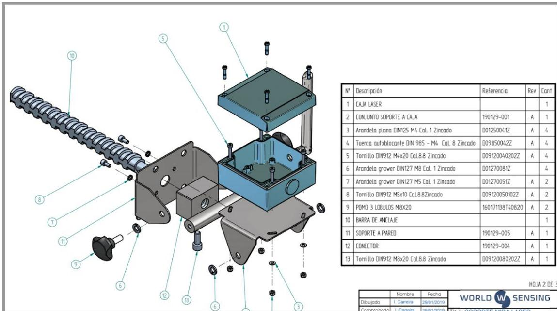
Swivel mounting bracket, exploded diagram
