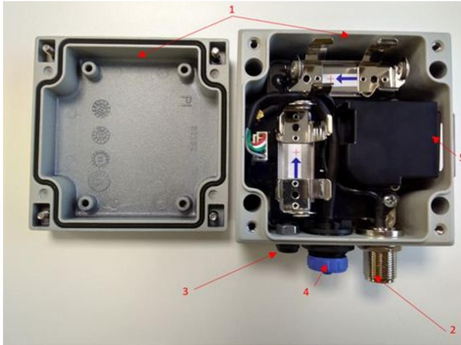
*Laser node and its labelled component parts*
