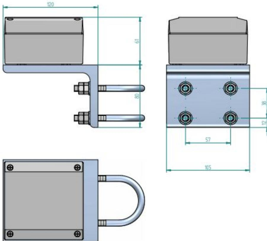
*Vertical mounting plate for pole mounting*
