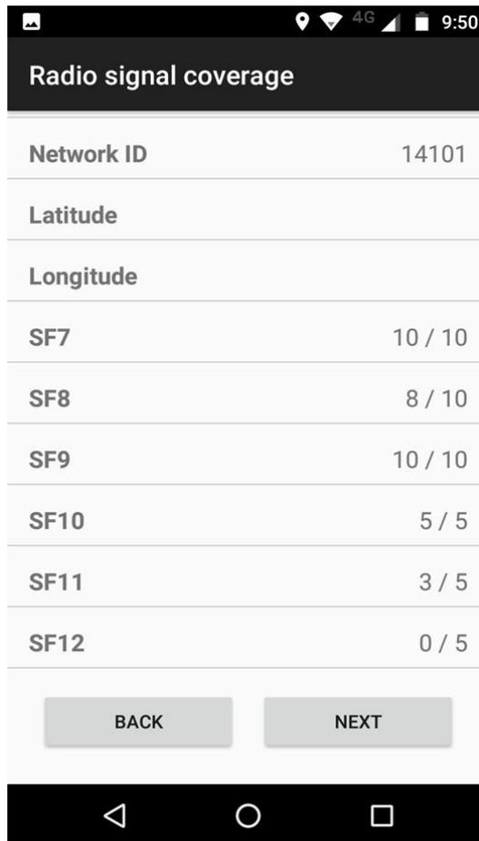
*Radio signal coverage test, Setup wizard*
