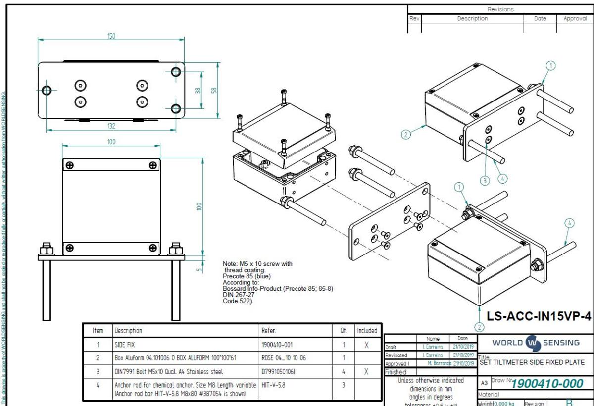
Fixed mounting for vertical surfaces, exploded diagram
