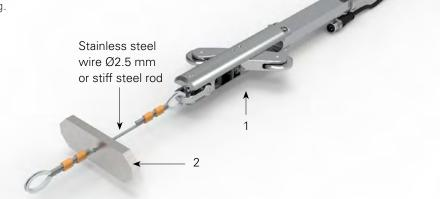
Continue with the other BH Profile probes untill completing the whole chain. All reference BH WROGIS In US position and cable at the upper BH Profile probe. Assemble the suspension system (2) according to the above draw (see also "Appendix 2"). Connect the upper cable with female connector to the male connector of the upper BH Profile probe.
