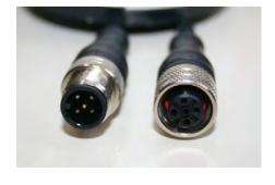
To obtain a correct connection align the key references. Do not strain or screw tightly to avoid damaging the connectors. Protection IP68 (1MPa) is guaranteed only with a good connection.
