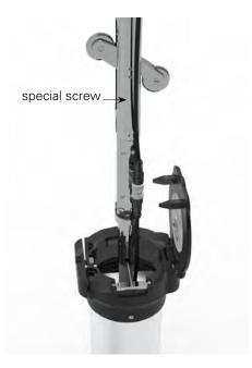
Connect the second BH Profile screwing the supplied special screw. Take care during the connection to the reference wheel that shall run in the reference keyway.
