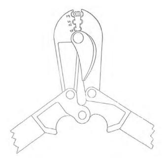
Plier for copper clamps mm 2, 2.5, 3. Use only for supplied copper clamps.
