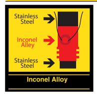
The core body of our Piezometer uses Inconel alloy instead of stainless steel. This type of alloy is well suited for service in extreme environments subjected to pressure and heat. The physical behavior of Inconel alloy enhances our VW Piezometer with a longer life and more stable data output.
