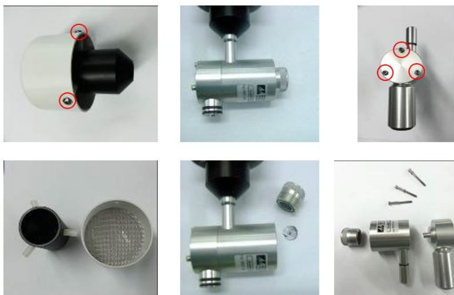
Figure 6-45 The TSP head and cyclone can be disassembled for cleaning.
