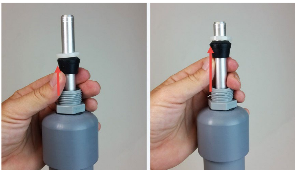
Figure 6-31 Create more length to the inlet by sliding the black rubber grommet up the tube.
