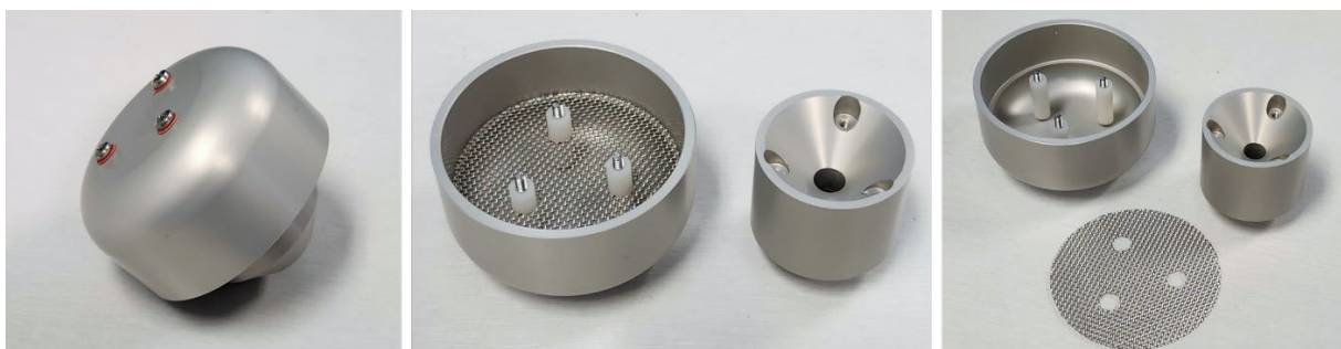
Figure 6-21 PCX TSP inlet disassembled for easy cleaning.
