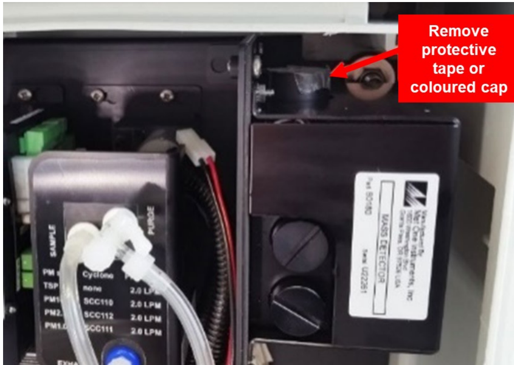
Figure 6-29 Remove the protective tape or cap from the PM inlet
