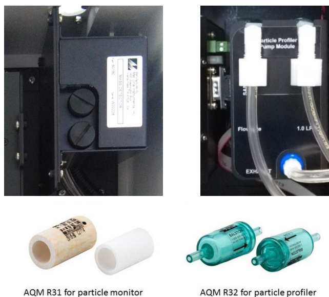
Figure 6-42 The Particle Nephelometer (shown on the left) requires AQS R31 and the Particle Profiler (shown on the right) requires AQS R32.
