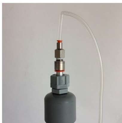
Figure 6-36 Positioning of the flow adapter when checking the flow rate on a Particle Profiler.
