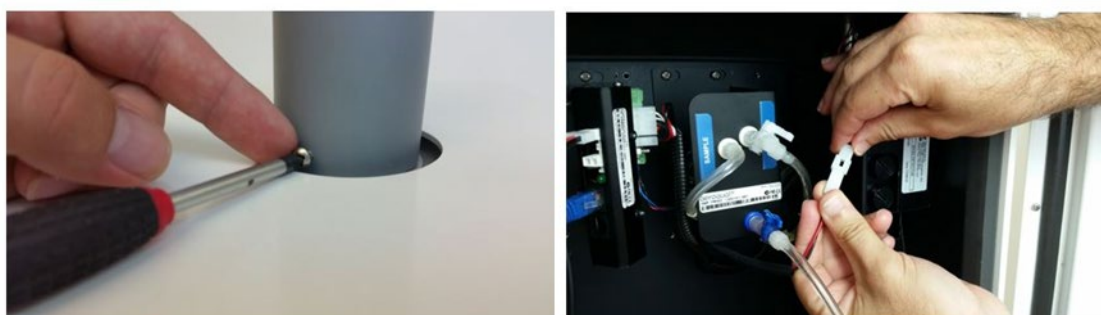
Figure 6-32 During field installation, secure the PM inlet using the retaining screws, then plug in the heater
