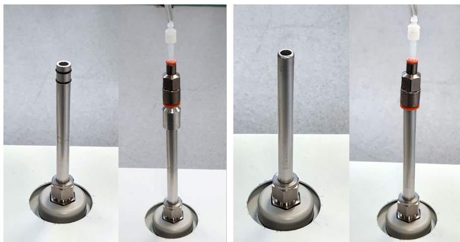
Figure 6-18 When checking the flow rate of the PCX replace the inlet with the adapter as shown. Left: V1.0 inlet with O-rings that requires an extra adapter. Right: V1.1 inlet without o-rings on the tube.
