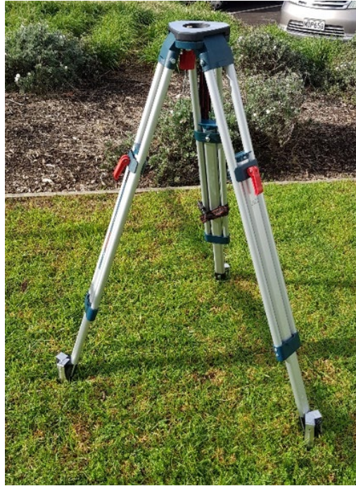
Figure 3-2 A tripod can be secured in the desired location using pegs
