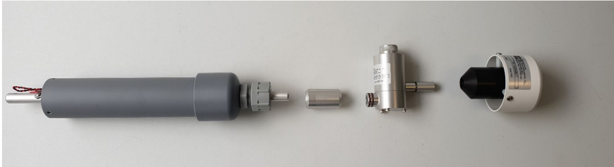
Figure 6-27 Particle sampling inlet parts including (L-R): inlet tube, cyclone adaptor, cyclone, TSP head.
