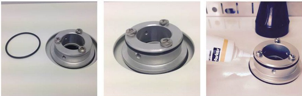
Figure 6-28 Add the O-ring and a small amount of lubricant.
