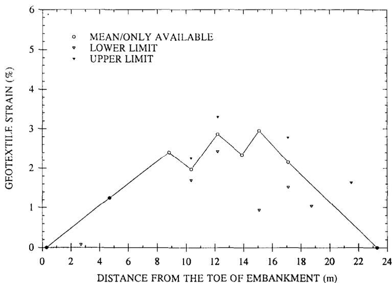
Fig. 18. Geotextile strain distribution at embankment thickness = 5.7 m (475 h).
