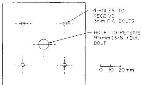
Fig. 6. Details of mechanical gauge reference point.
