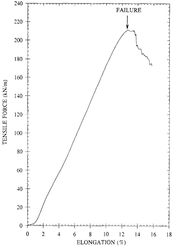
Fig. 7. A typical tensile force vs elongation plot.
