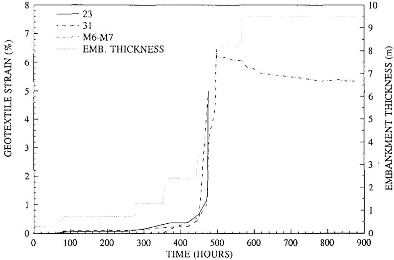
Fig. 11. Variation of geotextile strain with time for gauges 23, 31 and M6-M7.
