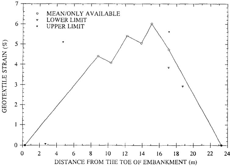
Fig. 19. Geotextile strain distribution at embankment thickness = 7.0 m (493 h).
