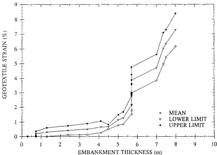
Fig. 14. Variation of geotextile strain with embankment thickness for gauges between 16.6 and 17.6 m from embankment toe.
