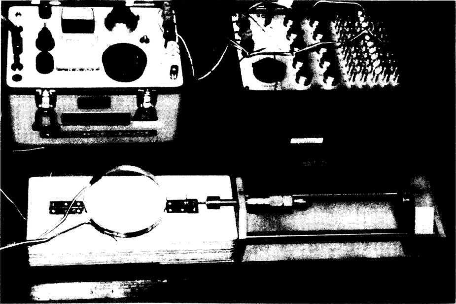
Fig. 5. Arrangement used for the calibration of electromechanical ring gauges.
