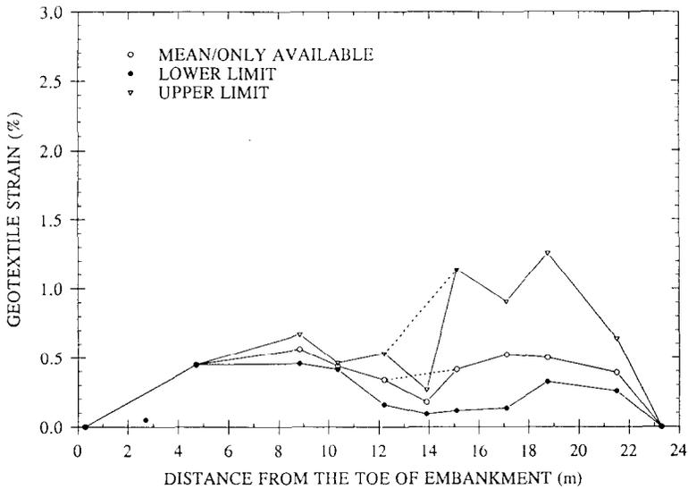
Fig. 16. Geotextile strain distribution at embankment thickness = 3.4 m (448 h).
