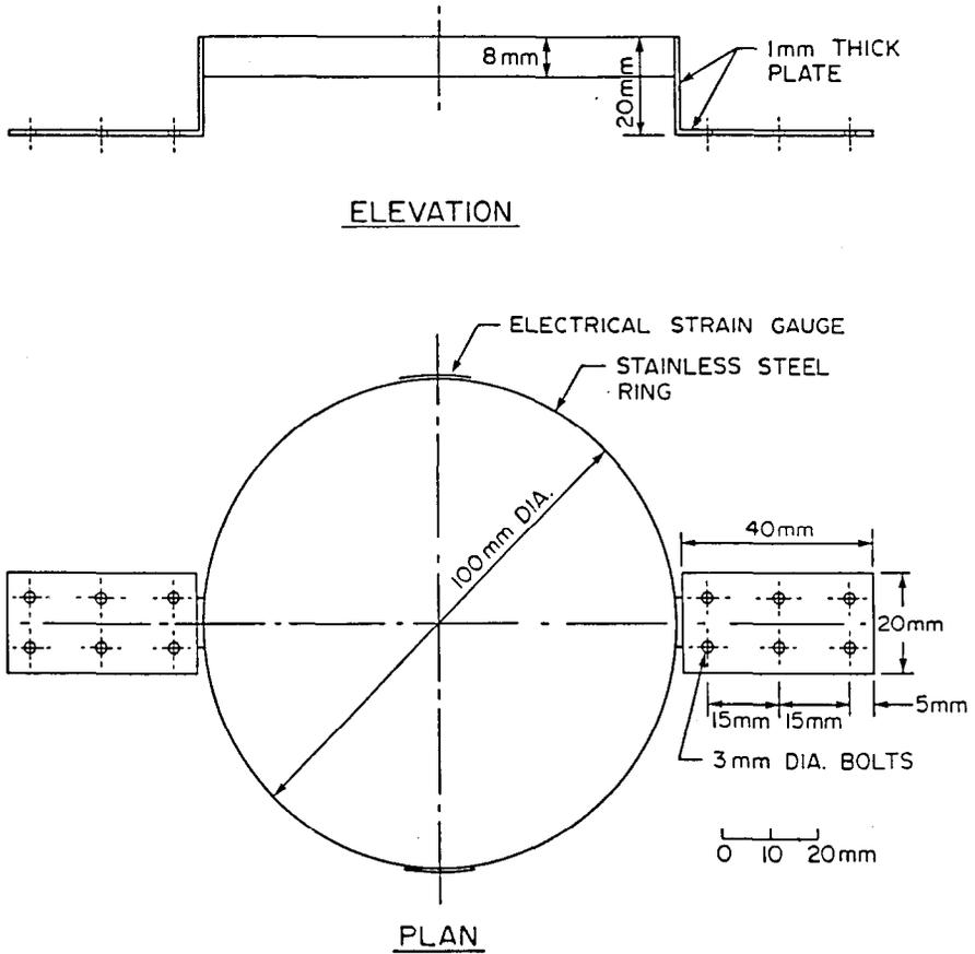
Fig. 4. Details of electromechanical strain gauge.
