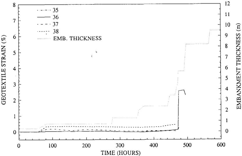
Fig. 12. Variation of geotextile strain with time for longitudinal gauges 35-38.
