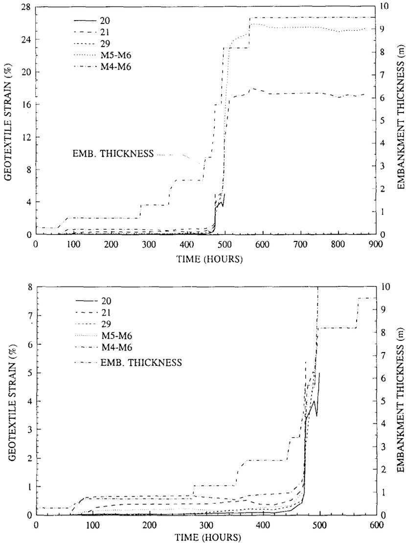
**Fig. 10.** (a), (b) Variation of geotextile strain with time for gauges 20, 21, 29, M5-M6 and M4-M6.
