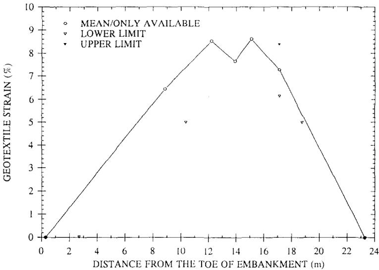
Fig. 20. Geotextile strain distribution at embankment thickness = 8.2 m (497 h).
