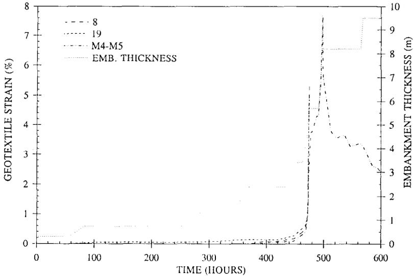
Fig. 9. Variation of geotextile strain with time for gauges 8, 19 and M4–M5.
