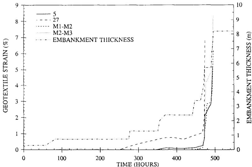
Fig. 8. Variation of geotextile strain with time for gauges 5, 27, M1-M2 and M2-M3.
