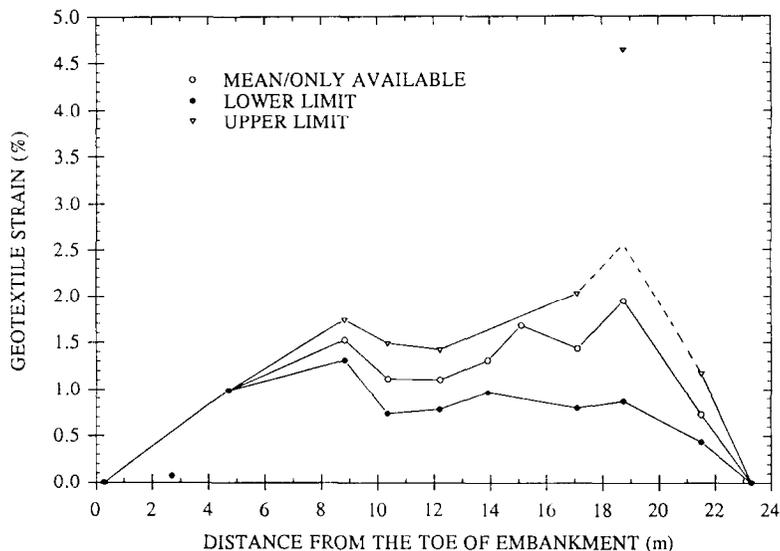
Fig. 17. Geotextile strain distribution at embankment thickness = 5.0 m (472 h).
