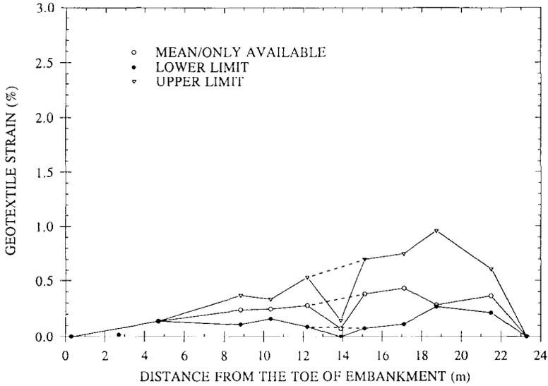
Fig. 15. Geotextile strain distribution at embankment thickness = 2.4 m (372 h).
