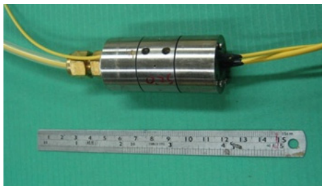
Figure 2. The FBG pressure transducer.
