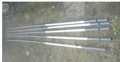
Figure 7. PVC pipes with FBG piezometers enclosed.
