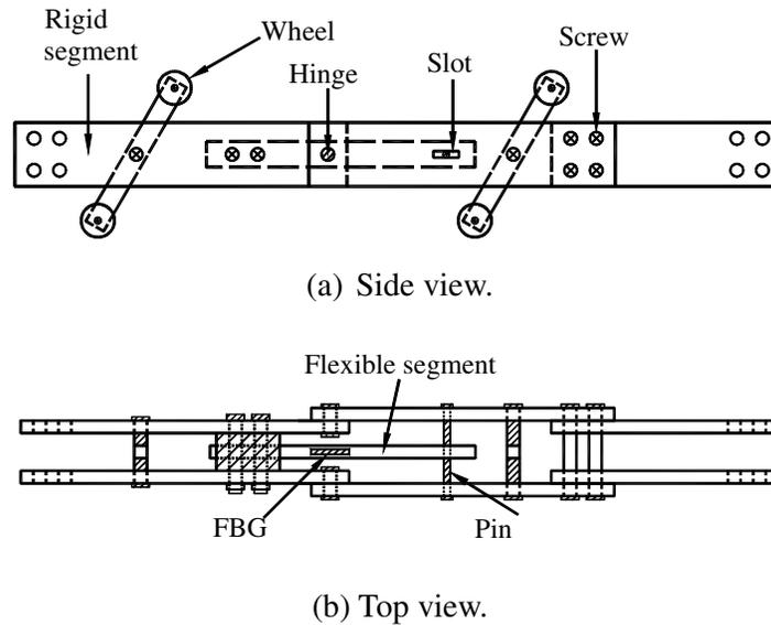
Figure 4. Schematic views of a single FBG-SD unit (from Ho et al., 2006).
