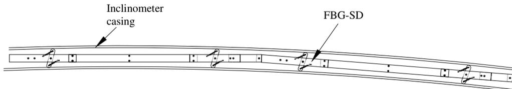
Figure 5. Rotation of FBG-SD caused by casing deflection (from Ho et al., 2006).
