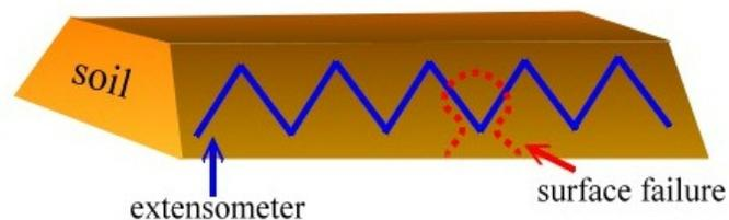
Figure 1 Layout of optic fibers on the slope surface to detect failure.
