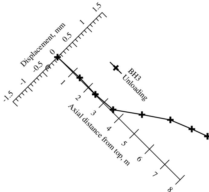
Figure 9. Displacement profile of BH3 after removal of 9.7m<sup>3</sup> of rock pile.
