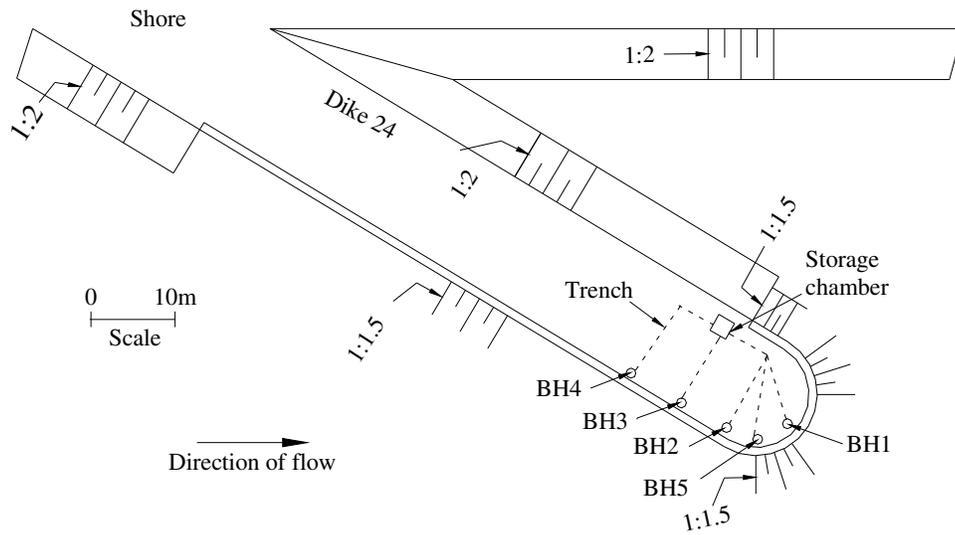
Figure 2. Plan view of Dike No.24.
