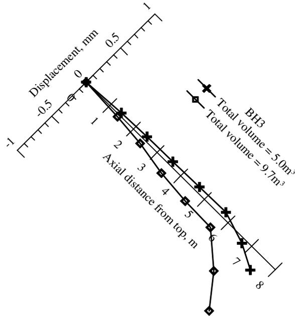
Figure 8. Displacement profile in BH3 from the first loading test.
