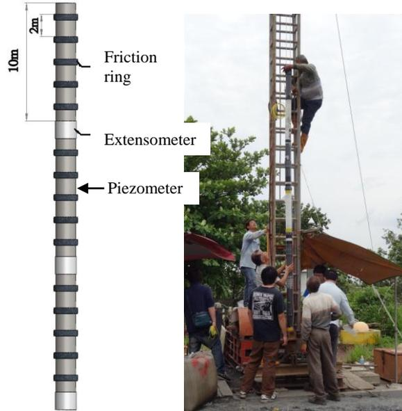
Figure 4 Field installation of the integrated FBG ground subsidence monitoring array.
