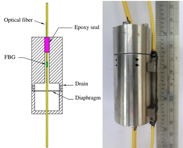
Figure 2. The FBG pressure transducer.
