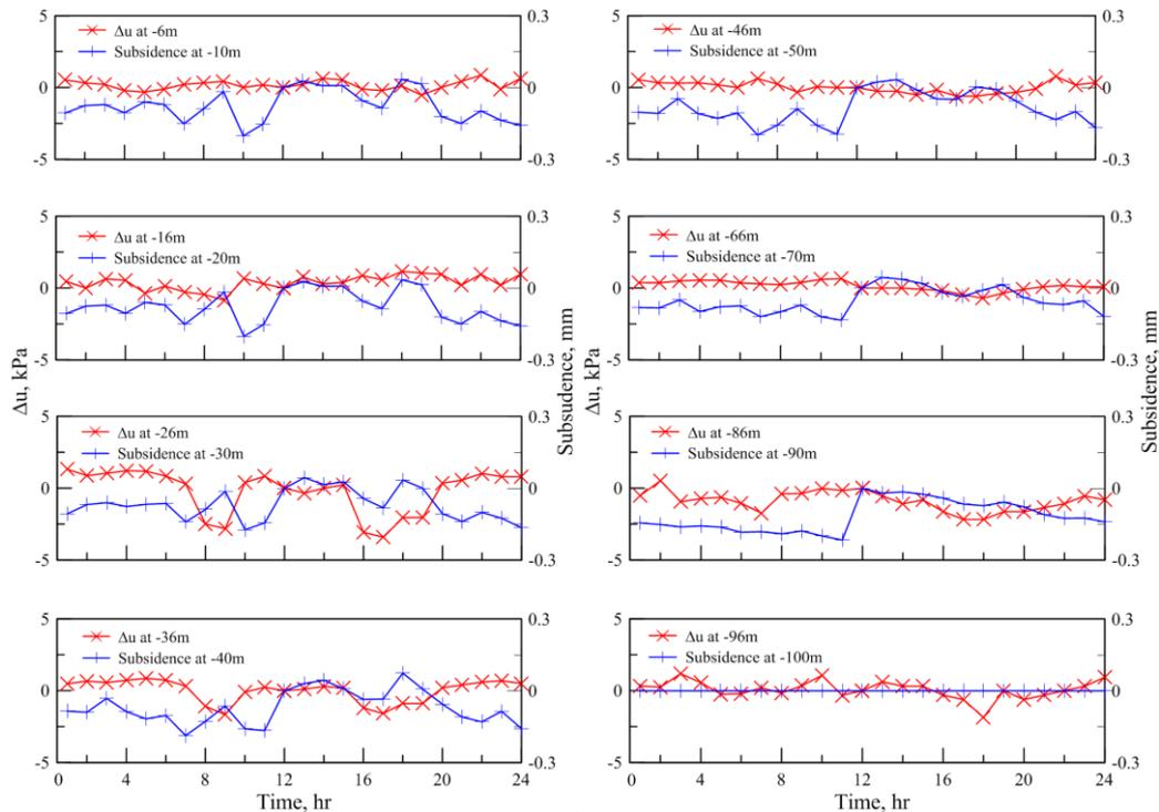
Figure 6. Time history of pore water pressure and ground subsidence within 24 hours.
