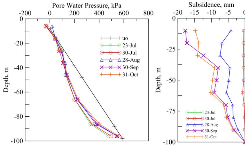
Figure 5. Pore water pressure and ground subsidence profiles.
