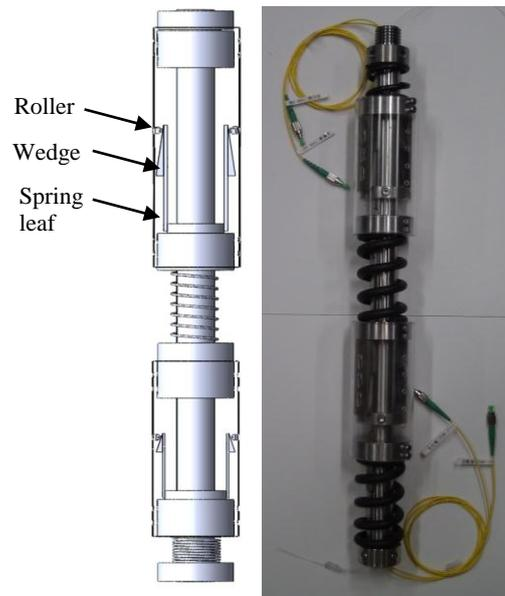
Figure 3. The FBG extensometer.
