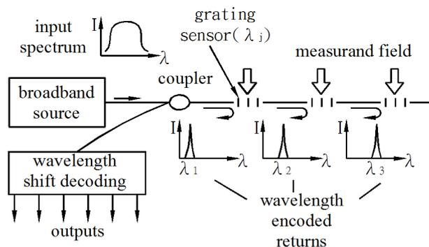
Figure 1. Schematic diagram of Fibre Bragg Grating (after Kersey [1]),
