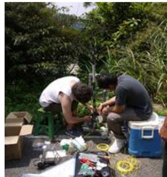
(b) Assembly and insertion of FBG-IPI
