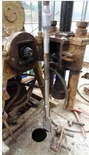
Fig. 18 The fully assembled  $\Delta$ DMT.
