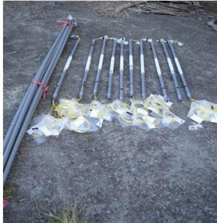
**Fig. 9 PVC pipes and those with FBG piezometers enclosed.**
