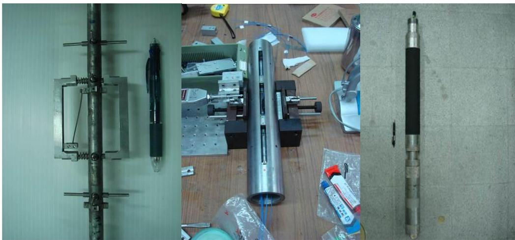
(a) Strain arms (b) Tube section (c) Fully assembled PMT
