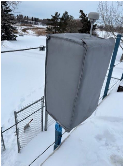
Fig. 7: The Dust Sentry deployed at the Henry Pirker station, showing the winterization jacket.
