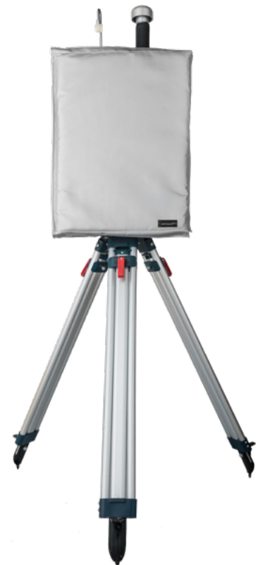
Fig. 1: Aeroqual AQS 1 with Winterization jacket.
