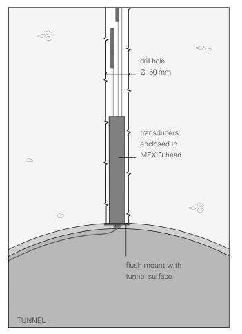
MEXID Required drill hole: Ø 50 mm (2"), Ø 75 mm (3") first meter Flush mount maximizes clearance Enclosed transducers
