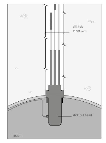
MPBX MULTIPOINT BOREHOLE EXTNSOMETER Required drill hole: Ø 101 mm (4"), Ø140 mm (5.5") first meter Stick out reduces clearance up to 510 mm Transducers installed at site
