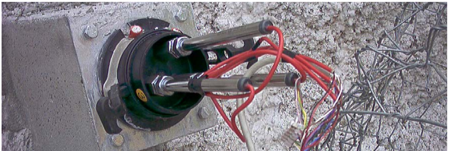
MPBX head with displacement transducers, installed on retaining wall
