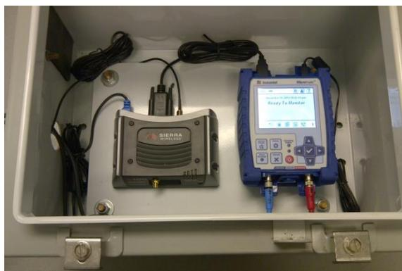
**Mounting Panel Installed in the Enclosure**
