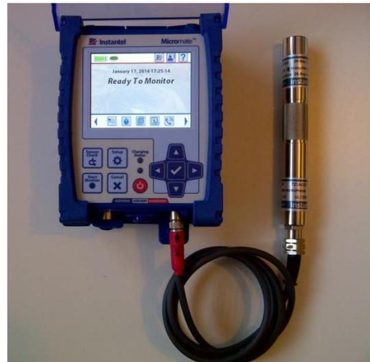
**Microphone Connected to the Micromate**
