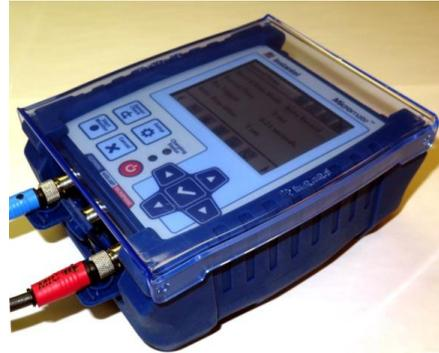
Micromate Installed in the Protective Boot
