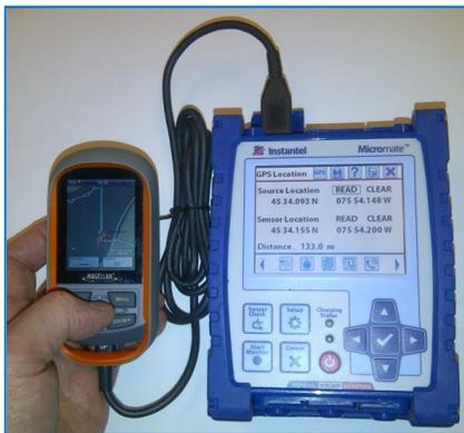
GPS Connected to the Micromate
