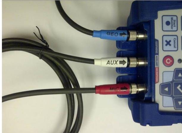
**External Trigger Cable Connected to Micromate**
