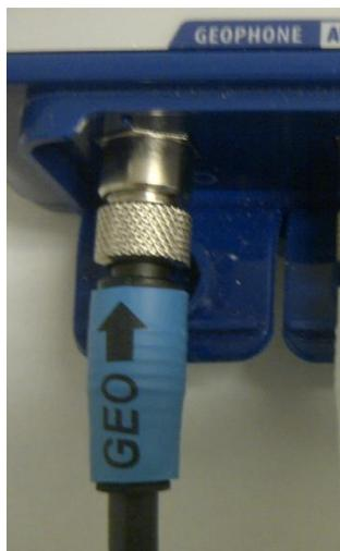
Geophone Connected to the Micromate
