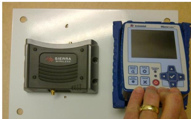
**Install the Micromate in the Protective Boot**
