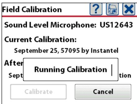
Micromate Calibrating Sound Level Microphone
