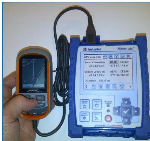
**GPS Connected to Micromate**
