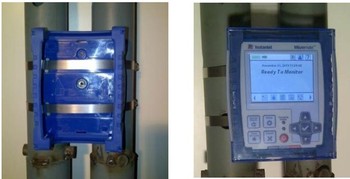
**Micromate Attached with Metal Straps**
