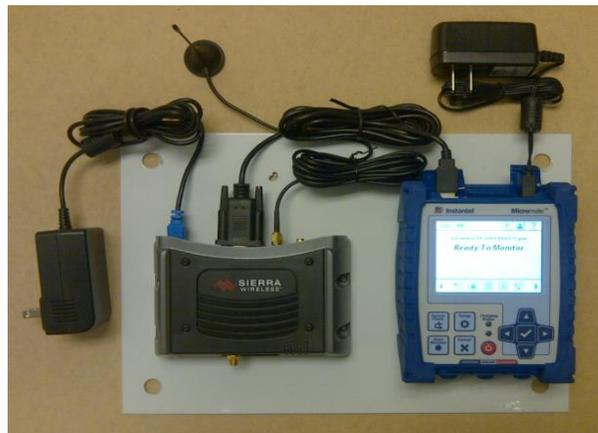
Placement of Modem, Micromate and Cables
