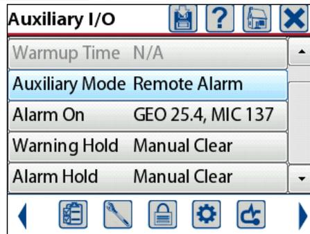
**Sample Auxiliary I/O Configured for a Remote Alarm**
