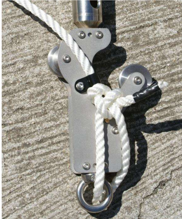
Figure 5: Polypropylene rope connected and secured to eyelet on the base of the bottom wheel assembly
