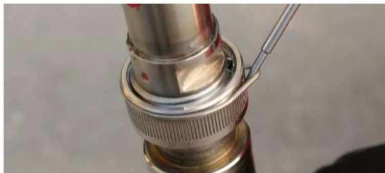
Figure 22: Retaining ring levered out of the recess using a screwdriver
