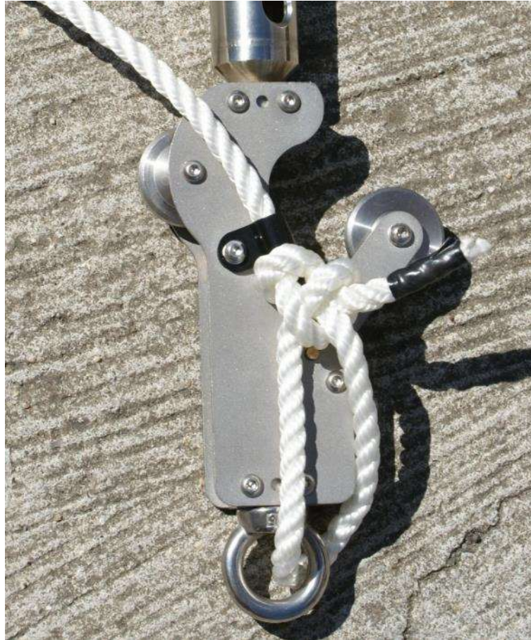
Figure 18: Polypropylene rope connected and secured to eyelet on the base of the bottom wheel assembly
