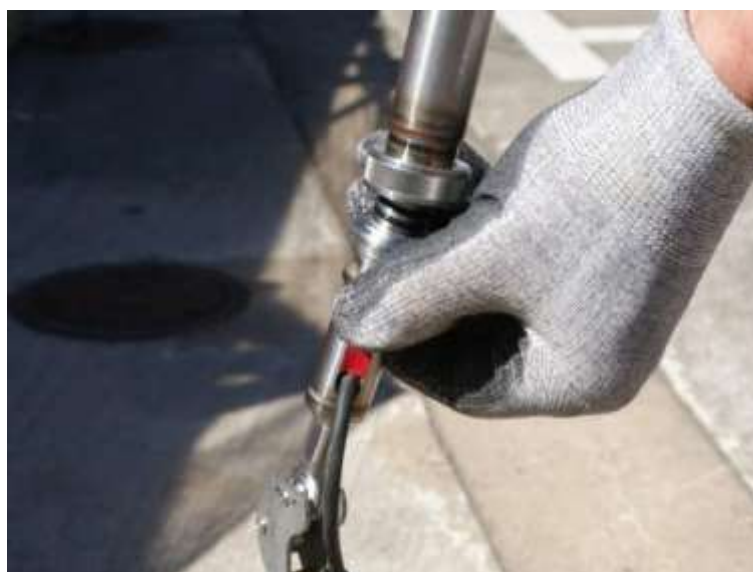
Figure 7: IPI male and female connectors being pushed together
