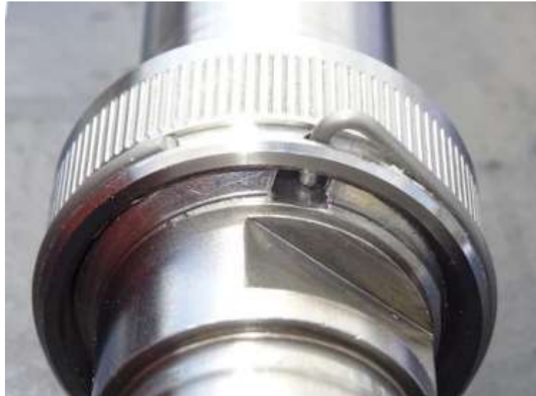
Figure 8: Retaining ring or "snap ring" engaged into recess, locking the threaded collar and stopping it rotating
