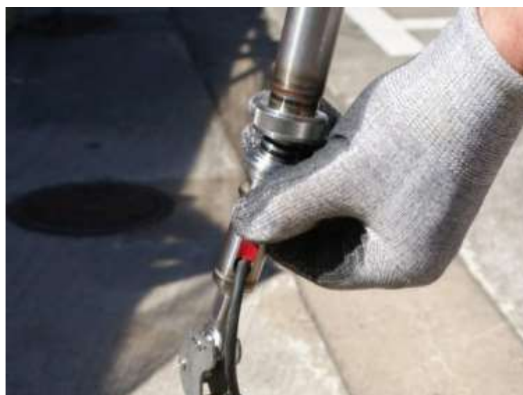
Figure 20: IPI male and female connectors being pushed together
