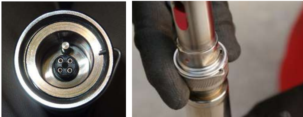
Figure 19: Alignment pin and marker dot
