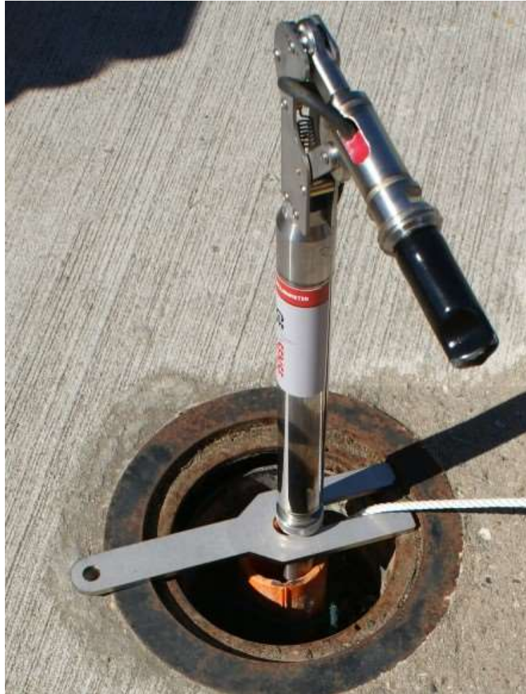
Figure 11: Installation fork locked off on the flats of the sensor, supporting the weight of the half installed string whilst the next sensor is prepared and added onto the top of the locked off sensor
