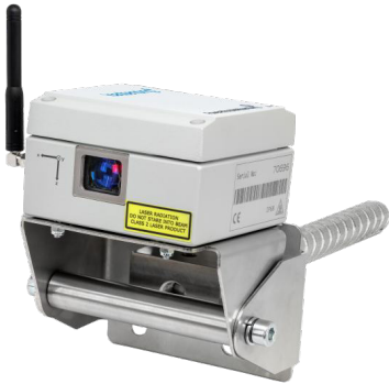
Fig. 5: LaserTilt90 on a swivel mounting bracket LS-ACC-LAS-SB attached to a WS-ACC-LAS-NSB-ADAP to be installed with a convergence bolt G3/8" male thread.
