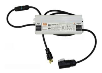
The Solar Rescue Charger is a portable, rugged, solar-compatible power system that supplies a 24V power source to a remote solar power kit. The sturdy aluminum case is built to withstand all weather elements. The system includes an AC input for 120/240VAC and outputs 24VDC over a weatherproof connector to charge the battery in your solar kit.
