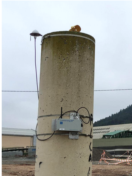
Figure 6: Installation of a base in a survey pillar. A prism for survey control has been installed on top of it and its position is being used as the base position for Loadsensing GNSS installation. The GNSS antenna has been installed within a certain distance from the radio antenna by using a 2,5 m cable
