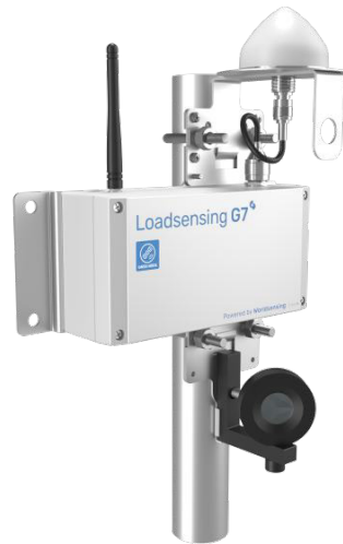
Fig. 2: Compact mount with u-bolts. Use the LS-ACC-BIG-HVP versatile mount plate and WS-ACC-U50 50mm U-bolts to secure the device to a 50mm pole. Attach the LS-ACC-ANT-HVP versatile mount plate for the GNSS antenna to the node mount plate for a compact setup. Add the LS-ACC-PRS-VP prism mount plate for prism installation. Not recommended for base stations.
