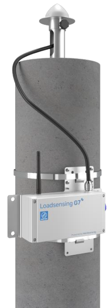
Fig. 2: Compact mount with U-bolts. Use the LS-ACC-BIG-HVP versatile mount plate and WS-ACC-U35 35 mm or WS-ACC-U50 50 mm U-bolts to secure the device to a 35 or 50 mm pole. Attach the LS-ACC-ANT-HVP versatile mount plate for the GNSS antenna to the node mount plate for a compact setup. Add the LS-ACC-PRS VP prism mount plate for prism installation. Not recommended for base stations.
