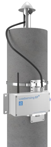
Fig. 3: Survey pole mount. Use the LS-ACC-BIG-HVP versatile mount plate to secure the device to a pole with metal clamps. Install the GNSS antenna on top of the pole using the LS-ACC-GNSS-RD 5/8-inch survey pole mount and the LS-ACC-GNSS-CL2 or LS-ACC-GNSS-CL3 cable extension. Suitable for base stations and rovers.
