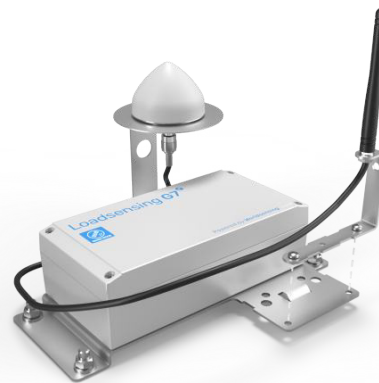
Fig. 4: Compact horizontal mount. Use the LS-ACC-BIG-HVP versatile mount plate to secure the device to a horizontal surface. Attach the LS-ACC-ANT-HVP versatile mount plate for the GNSS antenna to the node mount plate for a compact setup. Use the LS-ACC-ANT-LORA versatile LoRa mount plate and the LS-ACC-ANTS-G7 cable extension to position the LoRa antenna vertically.
