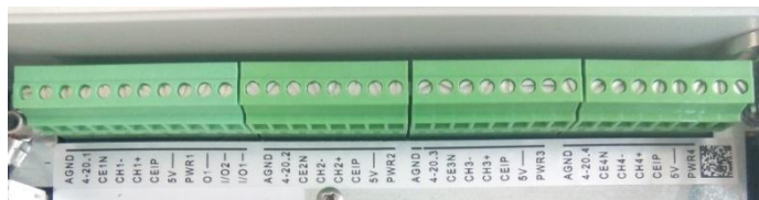
Image 1: Channels and connectors from the analog logger.
