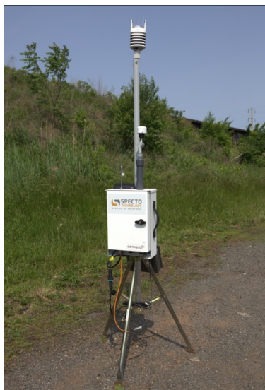
Real-time Perimeter Monitor (VOCs, “PM10” and Weather)
